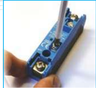
SA range with screw connection on inputs
